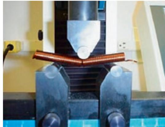
The wire test pieces are being tested with regard to the adhesive power of the wire coating.
